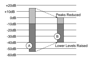
With Dynamic Range Control enabled, the full dynamic range (A) of the program is reduced (B).
